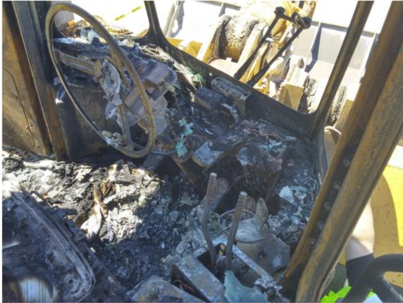
Fig. 2 – Damage of the operators cab from Hanford caterpillar loader fire
