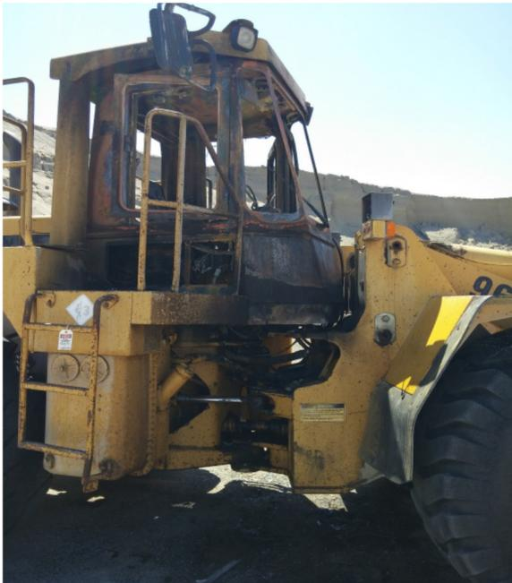
Fig. 3 – Char damage under the Hanford operators cab showing platform and ladder to the ground
