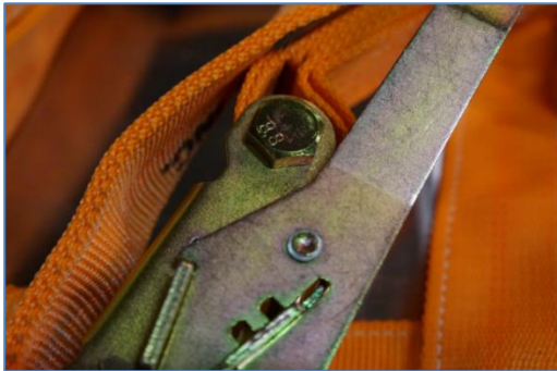
Figure 1. Image of S/CI bolt from Lessons Learned Report B-2017-PMA-PORTS-001
