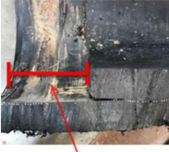
Figure 6: Pipe section is severely miss-stabbed.
