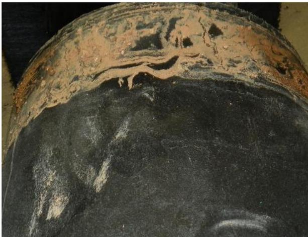
Figure 3: Dirt and mud in an area of the pipe and coupling where fusion between the HDPE should have occurred.
