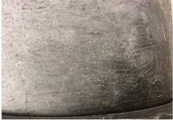
Figure 2: Coupling #1 Pipe surface was scraped.
