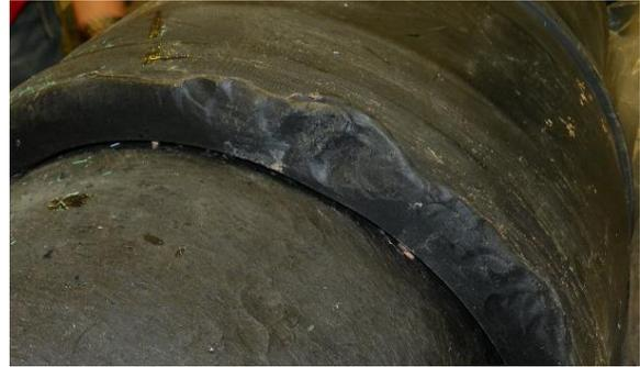
Figure 4: Hammer blows to the coupling indicate that pipe ends were not aligned and force was needed to install.
