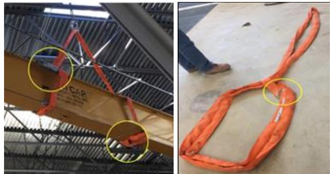
*Photos showing sling failure that caused girder to drop*
