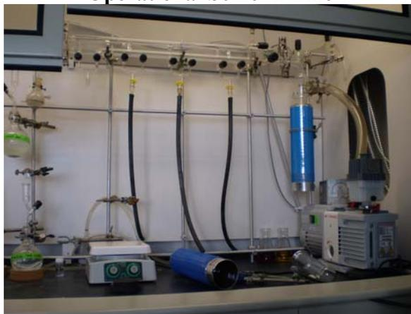
The depending black vacuum hoses deliver vacuum or inert gas. The pump on the far right delivers vacuum to the Schlenk manifold through the vacuum trap and its blue-jacketed Dewar. Not evident are a pressure-release bubbler or a ballast bulb.
